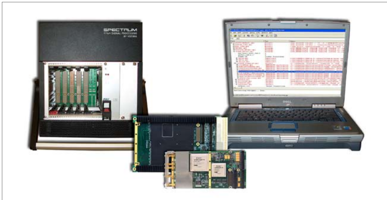
Spectrum Signal Processing's SDR-4000 configured with an SCA operating environment composed of GHS' Integrity RTOS, CRC SCARI++ Core Framework and OIS' ORBexpress
